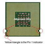
The surface of LGA 775 CPU Remember to apply some thermal paste on it for better heat dispersion.
